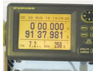
When the boat crossed the equator line the instrument panel showed we were at latitude 0.00.000.
